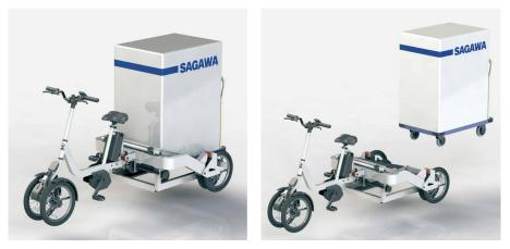
The towing section of the Trike Cargo vehicle attaches directly to a hand cart, and can be detached again with a single touch of a button (picture at right).
